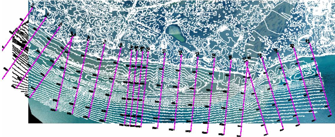
Figure 4. The bathymetry south of Bakkafjara as measured in 2002. The aerial photograph in the background is from 2002
