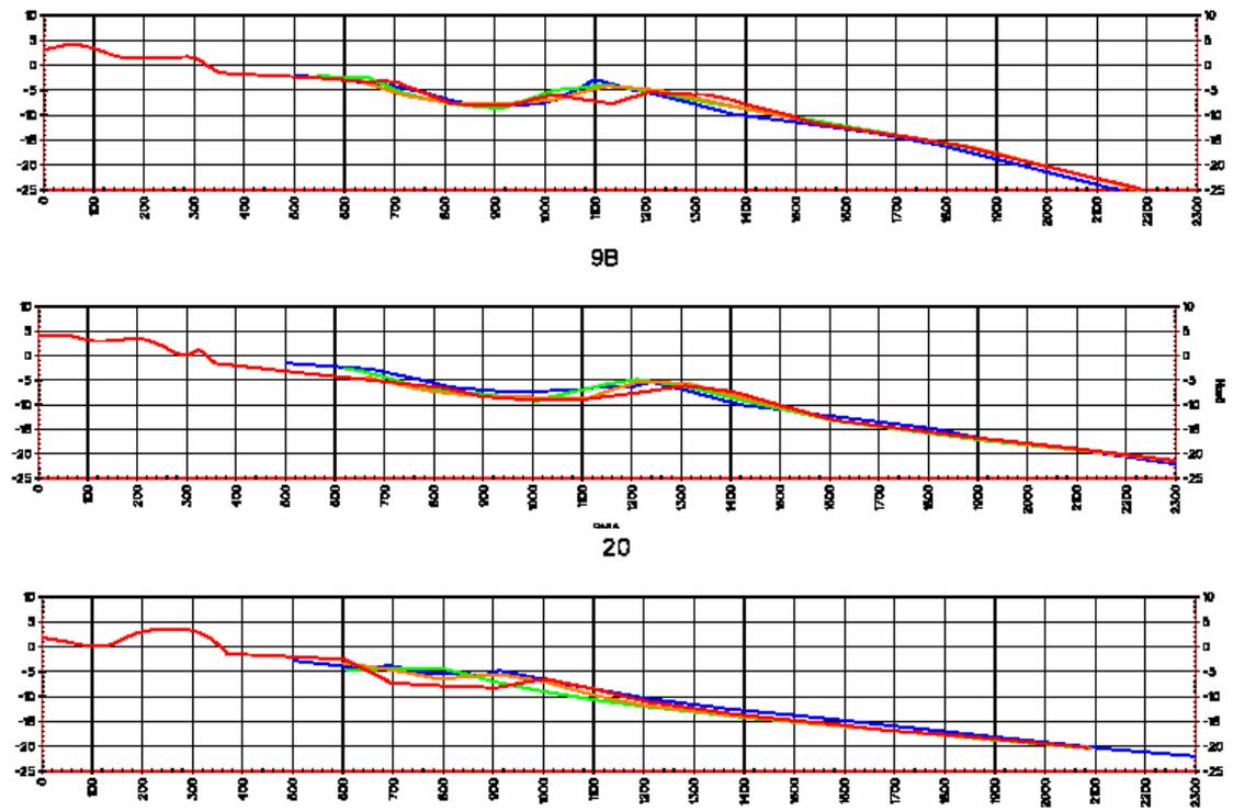
Figure 5. Bed elevations as measured in 1973, 2002, 2003 and 2004. The location of the lines is shown on fig. 4.
