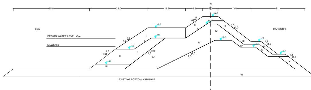
Figure 18. Bakkafjara berm breakwater. Class I: 20 -30 tons, Class II: 10 – 20, Class III: 4 – 10 tons, Class IV: 1 – 4 tons, Class V: 0.1 – 1 tons. Class VI: Scour protection of quarry run, 3 m tick.  $H_s$ , design = 7.0 m, a statistically stable berm design.
