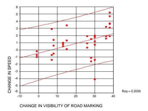
Figure 7.7 - Relationship between the change in the visibility of road markings and the change in the mean travel speed level.
