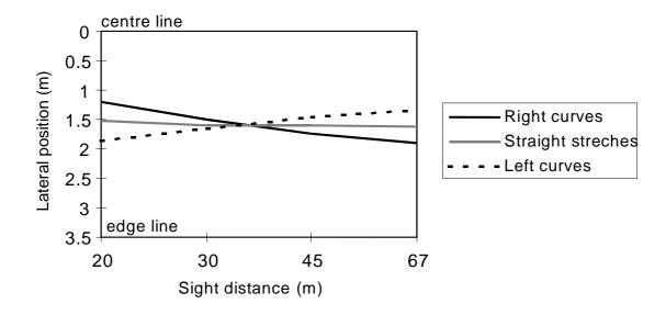
Figure 6.9 - Mean lateral position for right and left curves and straight stretches at the condition of cruise control.
