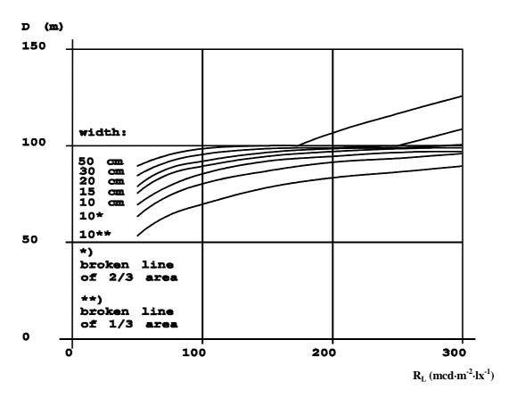
Figure 5.2 - Visibility distance (D) for edge lines in low beam illumination.
