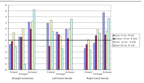
Figure 7.6 - Change in the mean travel speed by road marking type.
