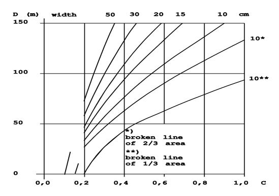
Figure 5.6 - Visibility distance (D) for longitudinal road markings in typical road lighting for traffic routes (1  $cd \cdot m^{-2}$  of road surface).
