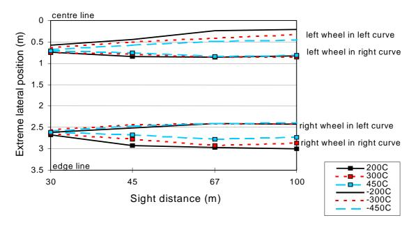
Figure 6.13 - Extreme lateral position of the wheel in the curves with clothoids at the condition of free choice of speed.
