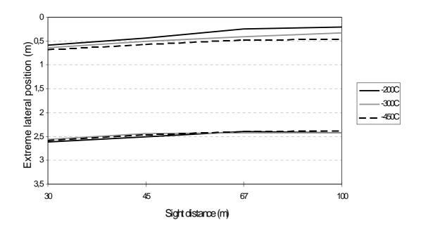
Figure 6.17 - Extreme lateral position of the wheels in left curve with clothoid at free choice of speed.
