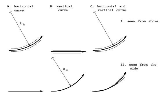
Figure A4.3 - Illustration of horizontal and vertical curve.
