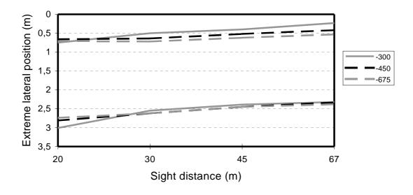
Figure 6.21 - Extreme lateral position of the wheels in left curve without clothoid at 90 km/h.
