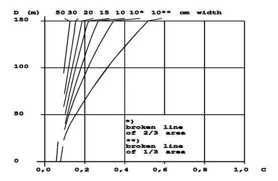
Figure 5.5 - Visibility distance (D) for longitudinal road markings in full daylight (1.000 cd·m<sup>-2</sup> of road surface).
