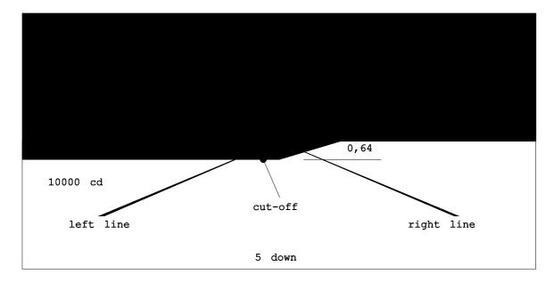
Figure A4.4 - Intensity distribution of the low beam (shown for right-hand traffic).
