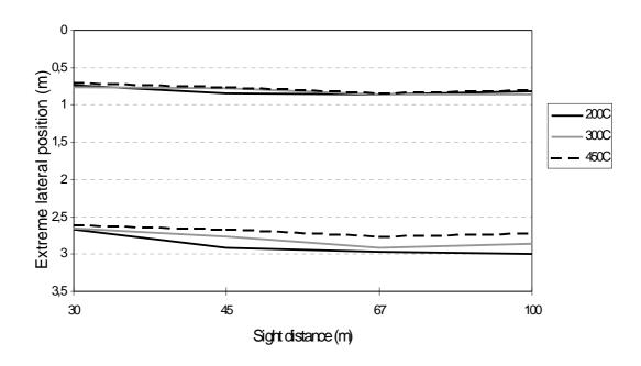
Figure 6.16 - Extreme lateral position of the wheels in right curve with clothoid at free choice of speed.
