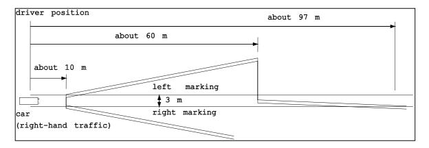
Figure D.1 - Reach of the cut-off of low beam headlamps for a passenger car driving in a 3 m wide lane.
