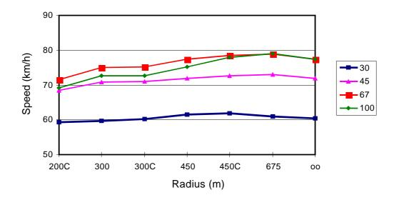
Figure 6.4 - Mean speed in curves and on straight stretches (C is for transition curves and oo is for straight sections).
