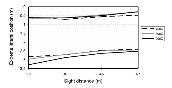
Figure 6.23 - Extreme lateral position of the wheels in left curve with clothoid at 90 km/h.
