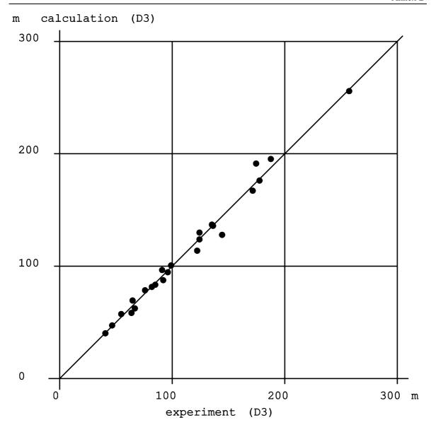
Figure B.5 - Comparison between experimental and calculated visibility distances
