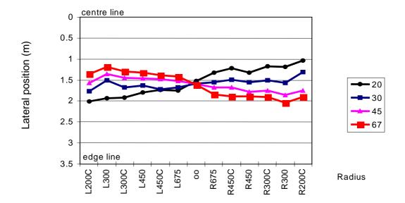
Figure 6.10 - Lateral position in every curve at the condition 90 [km/h] for different levels of sight distance.
