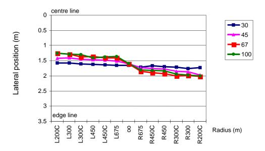
Figure 6.7 - Lateral position in every curve at the condition of free choice of speed at the four levels of sight distance.
