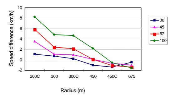
Figure 6.5 - Difference of mean speed on straight stretch and in curves at four levels of sight distance.
