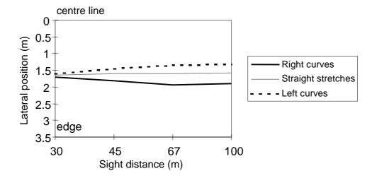
Figure 6.6 - Mean lateral position for right and left curves and straight stretches at the condition free choice of speed.
