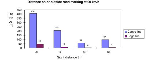
Figure 6.26 - Distance driven on, or outside, road marking at 90 km/h
