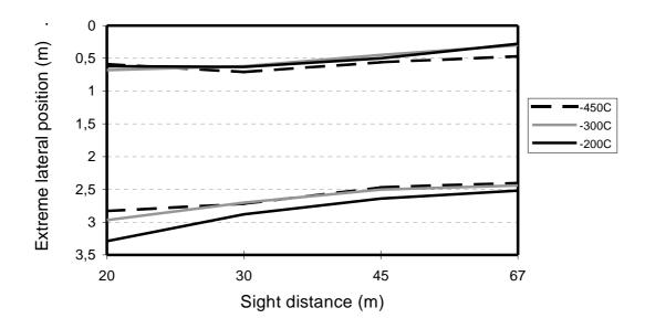
Figure 6.22 - Extreme lateral position of the wheels in right curve with clothoid at 90 km/h.
