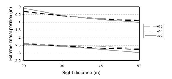
Figure 6.20 - Extreme lateral position of the wheels in right curve without clothoid at 90 km/h.
