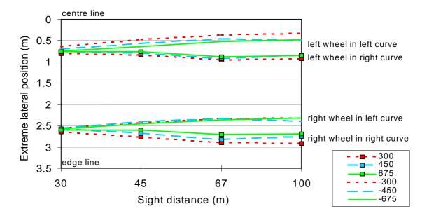
Figure 6.12 - Extreme lateral position of the outside wheel in curves without clothoids at the condition of free choice of speed.
