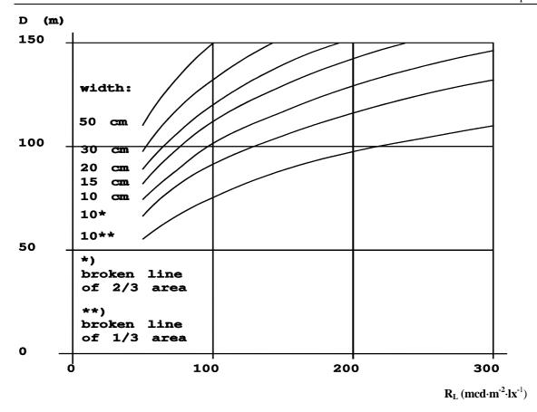
Figure 5.1 - Visibility distance D for longitudinal road markings in high beam illumination.
