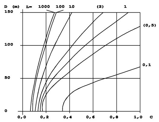
Figure 5.4 - Visibility distance (D) for a continuous road marking of 10 cm width in uniform illumination.
