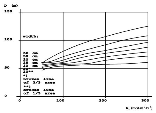
Figure 5.3 - Visibility distance (D) for centre lines in low beam illumination.
