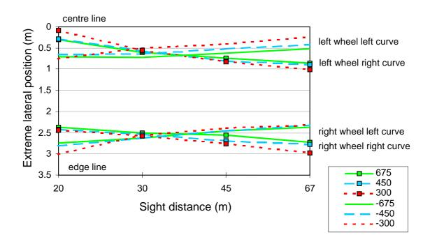
Figure 6.18 - Extreme lateral position of the outside wheel in curves without clothoids at the condition of cruise control.
