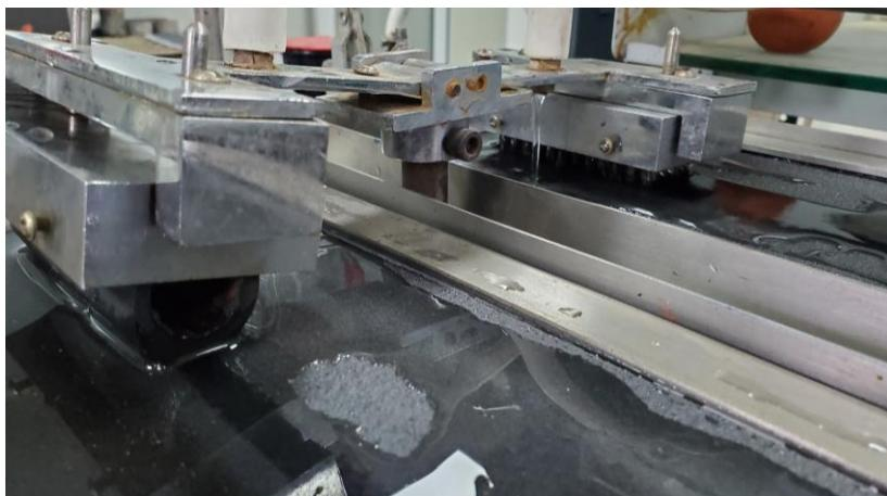
Metal Brush Abrasion, Coating Test
