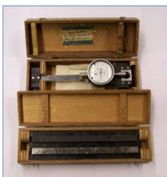
Figure 3-5: A strain gauge and equipments to measure creep.
