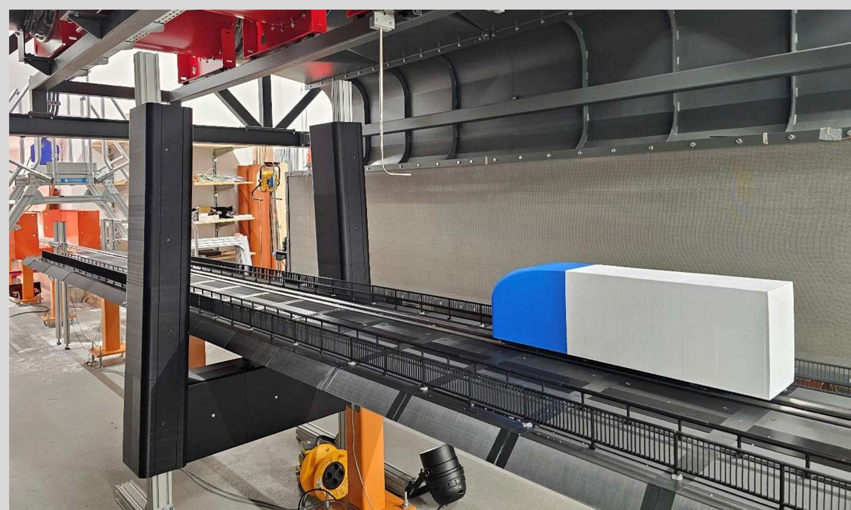
Figure 6: The model in the wind tunnel test section.
