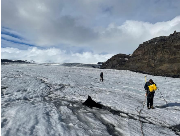
Figure 1. Conducting the radio-echo sounding survey to measure ice thickness on Sólheimajökull, May 2023. Photo by Greta Wells.
