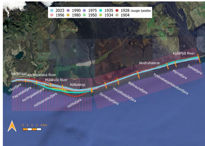
Figure 1. A map that shows all coastlines that extend over the research area along with the profiles set up to calculate changes in coastline location and volume. Each dot on the map is where the profiles intersect the line of each mapped coastline.
