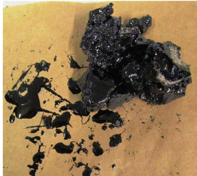
According to the visual inspection, the Road 1-K8 Section 11070 was the worst material; such surface dressing is extremely weak because of the very low viscosity of the binder causing significant binder bleeding. The surface dressing could not even take the own weight of the aggregate particles.
