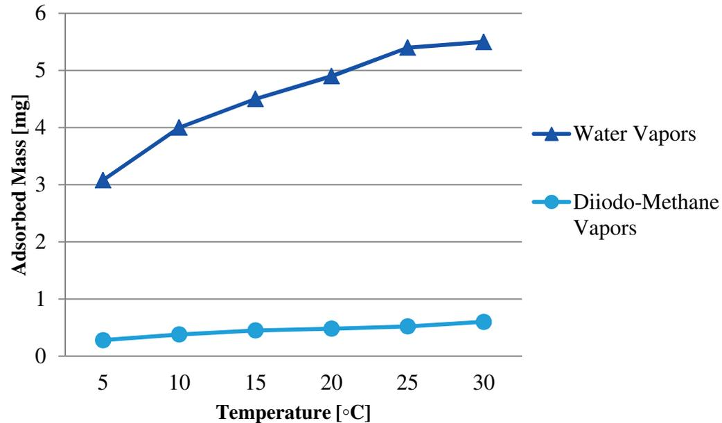
An increment of temperature or  $P/P_o$  (ratio between partial pressure and equilibrium pressure), leads to an increase in mass adsorbed at the stone surface. In case of water vapors, this mass increase was dominant as compared to the diiodo-methane vapors.
