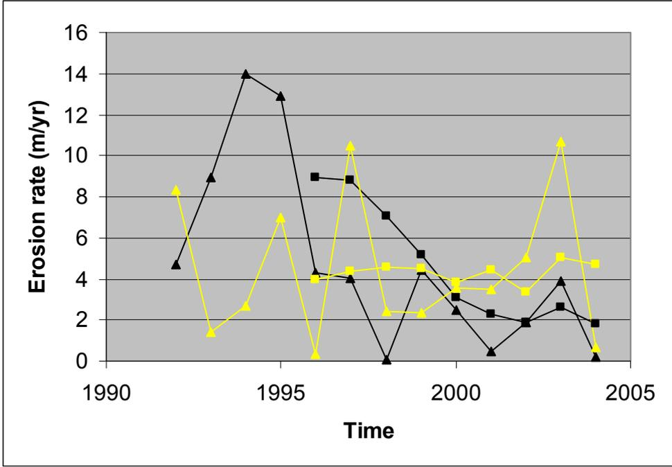
Figure 6b. Erosion rate of the steep bank 1200-2000 m west (black) and 1000-1800 m east (yellow) of Jökulsá. The triangles are yearly measurements and the squares are 5-year averages.
