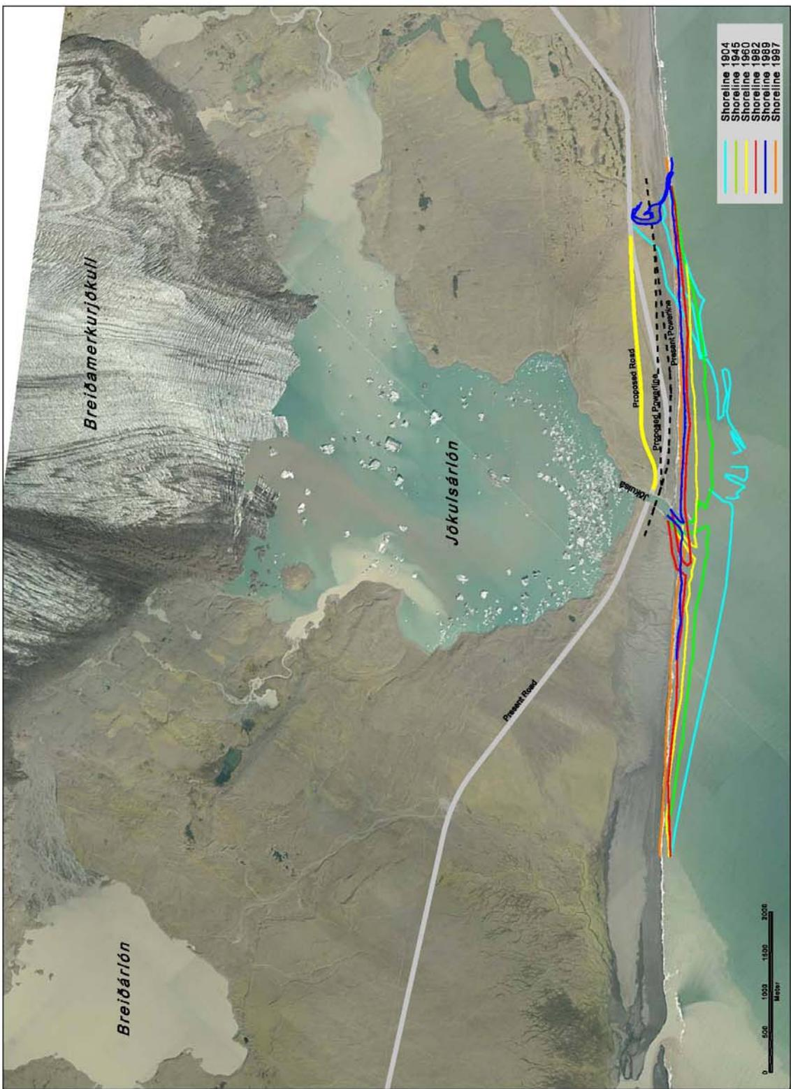
Figure 4. Shoreline changes at Breiðamerkursandur. Also shown is the present road / powerline and a proposed new road / powerline alignment east of Jökulsá. The aerial photograph in the background is from 2003.
