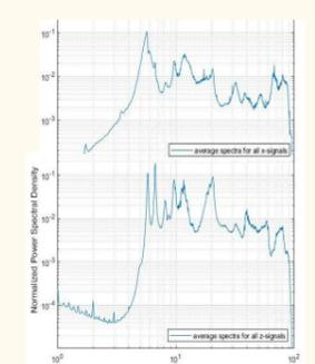
August - PSD plots, normalized with respect to the variance, showing the average for all recorded signals for each direction, as a function of frequency.
