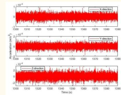
Time series recorded during the night in August 2019, showing a 90 sec segment of very stable low amplitude ambient noise.
