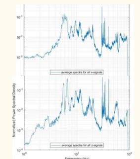
July - PSD plots, normalized with respect to the variance, showing the average for all recorded signals for each direction, as a function of frequency (in a log-log scale).
