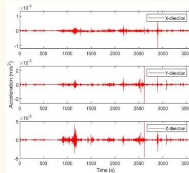
Time series example from accelerometer #3 in July 2019, showing spiky ambient excitation due to some undefined action on the bridge.
