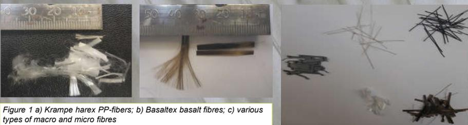
Figure 1 a) Krampe harex PP-fibers; b) Basaltex basalt fibres; c) various types of macro and micro fibres
