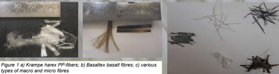
Figure 1 a) Krampe haxex PP-fibers; b) Basaltex basalt fibres; c) various types of macro and micro fibres
