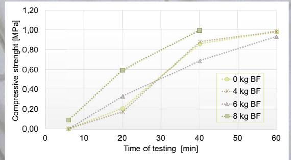
Figure 2: Comparison of early age compressive strength gain of sprayed concrete with 0, 4, 6 and 8 kg of basalt fibres tested by penetrometer.
