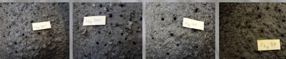
Figure 3: Images of the surface of test samples with various dose of basalt fibres content.
