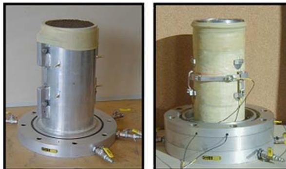
**Figure 2. Preparation of the specimen. a) Fully compacted specimen in the split cylinder; the outer part of the anchors can be seen sticking out of the cylinder. b) A specimen with the mounted displacement transducers.**
