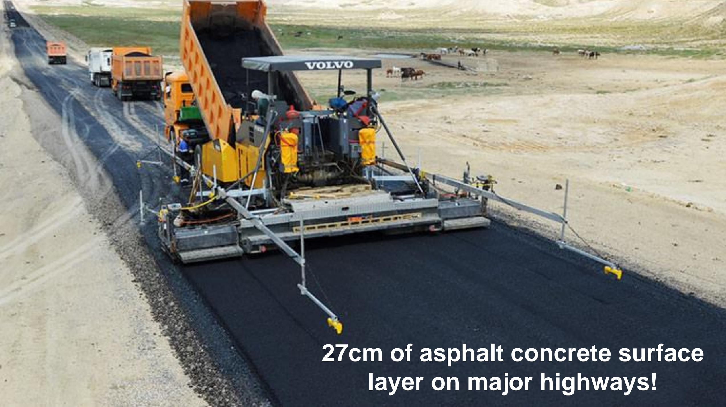
**27cm of asphalt concrete surface layer on major highways!**
