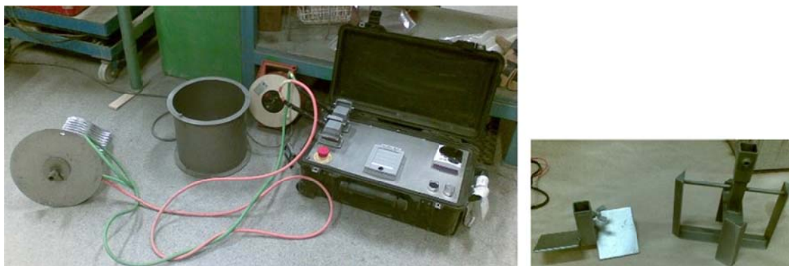
Figure 2: To the left is the ConTec Rheometer-4SCC. To the right are the two impeller systems. The larger impeller (the most right one) is the standard unit, while the smaller (on the left) is used to measure the RSI value.
