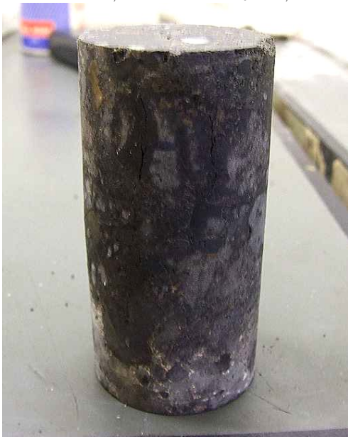
Sample nr. 16: Sandstone Failure at: \sigma_1 = 28,624 MPa and \sigma_3 = 0,891 MPa
