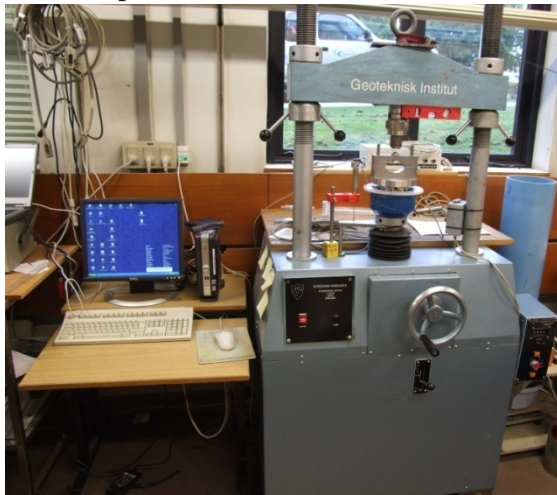
Figure 6-10: Test setup for Brazil test, includes a loading frame, a data logger, a load cell, a vertical strain gauge and a computer.
