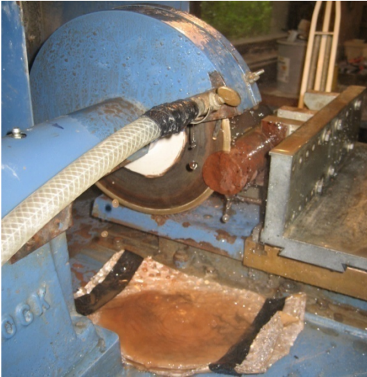
Figure 6-7: Siltstone waste away during cut off
