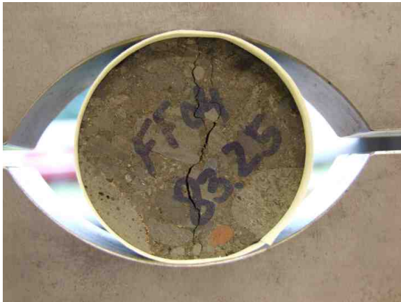
Sample nr. 20: Sandstone, \sigma_t = 1,22 MPa.
