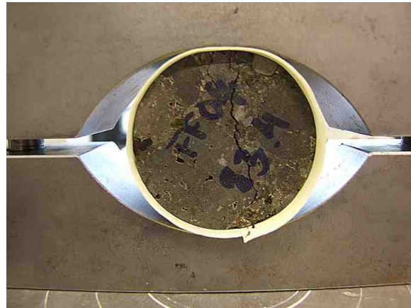
Sample nr. 21: Sandstone, \sigma_t = 1,53 MPa.
