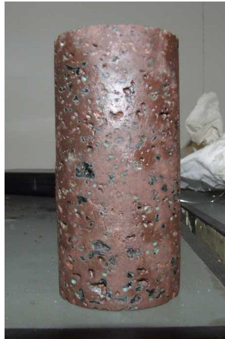
Sample nr. 14: Scoria Failure at: \sigma_1 = 25,123 MPa and \sigma_3 = 1,432 MPa
