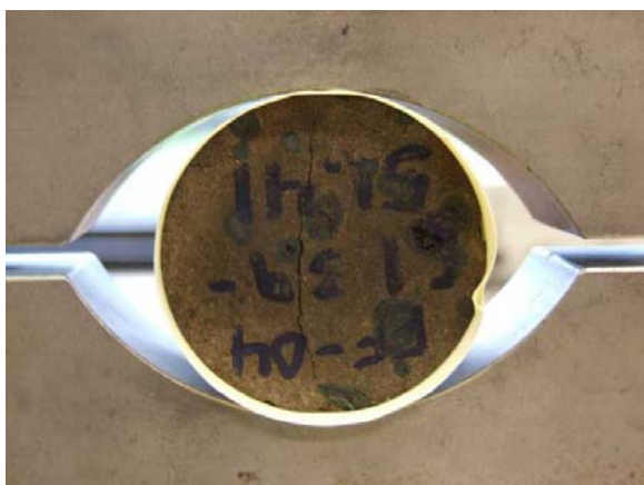
Sample nr. 36: Olivine t tholeiite, \sigma_t = 1,11 MPa.
