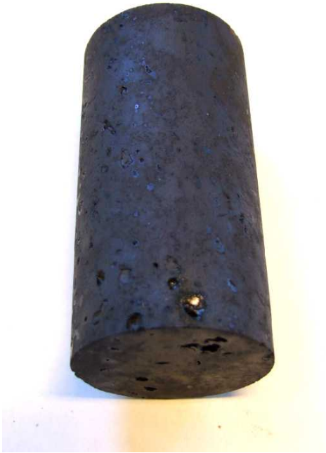
Sample nr. 3: Scoria Failure at: \sigma_1 = 25,346 MPa and \sigma_3 = 1,456 MPa
