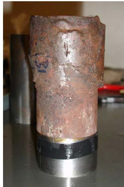
Sample nr. 5: Scoria Failure at: \sigma_1 = 6,321 MPa and \sigma_3 = 0,504 MPa
