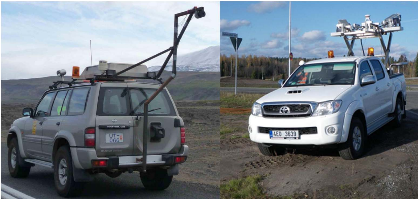
Everyman's RDLS Laser scanner survey vehicle (left) and a high precision Quantum 3D laser scanner survey vehicle (right) used in ROADEX surveys
